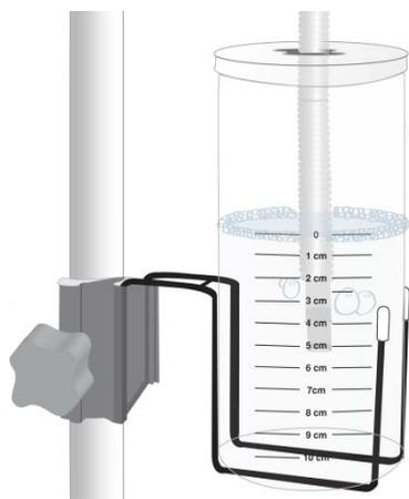
Attach the 10mm corrugated tube with air diffuser to the expiratory limb of the continuous flow breathing circuit. Insert the tube through the center hole to the desired depth with the flow rate on. Slide the tube sideways into the notch that secures the tube in position. The depth the tube is submerged in cm = positive airway pressure in cmH<sub>2</sub>O. Verify the pressure with an inline pressure gauge and adjust the depth as needed. Apply the protective cover to the top of the canister.
