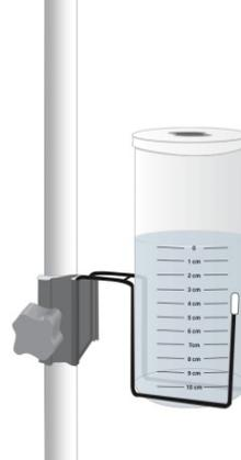
Fill the canister with water to the 0 cm line
